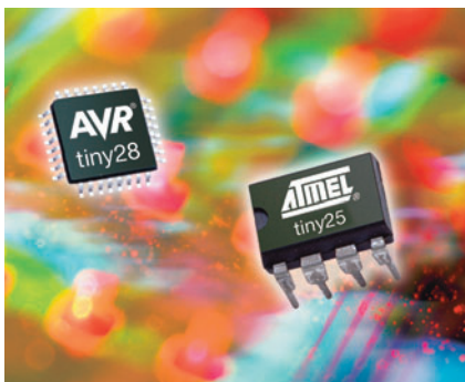
Fig.1: Atmel's AVR series: a 50ns instruction cycle time from a 20MHz clock
