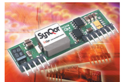
Fig.5: SynQor's vertically-mounted NiQor regulators deliver up to 15A
